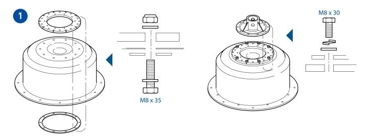
Turn the bowl top over and lower it on to the bowl base. Holes for mounting the mixer paddles are located in the hood top and the drive hub, where 2 bolts have been left out. Use Detail A as a guide for the arrangement of the mounting holes when aligning the screws to fix the bowl top together.
